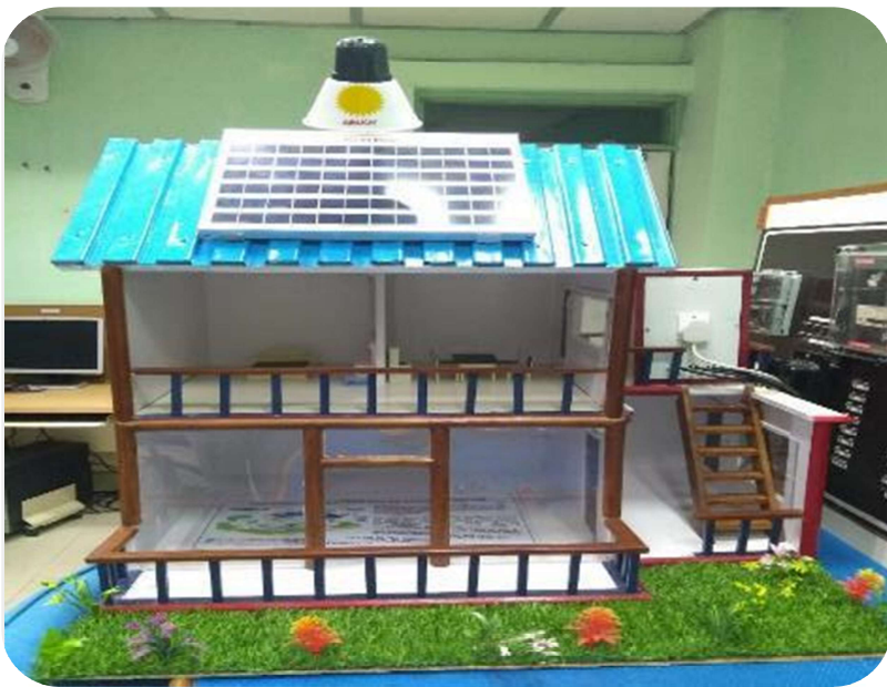
Working model residential rooftop solar energy system
