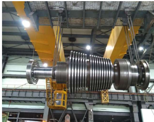
Refurbished IP turbine
