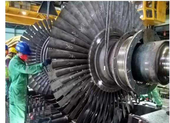
Servicing LP turbine
